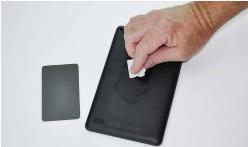
8. Remove the protective backing from the tablet adapter. Find the center of the tablet, then line up the adapter so that it is evenly spaced. Place one edge of the adapter against the tablet as shown. Once you have confirmed the adapter is centered, rest the adapter against the tablet and press into place.
